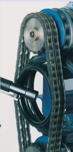
Roll-Ring® chain tensioners in one of our test rigs
